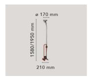
adjustable stem with telescopic head. On the cable there is the electronic dimmer which allows the regulation of light brightness.
