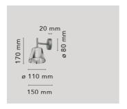
Gray painted die-cast aluminum diffuser and lamp support. Gray painted, injection-molded polycarbonate wall fitting and rose.
