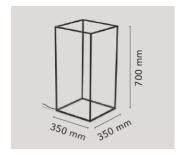
Floor lamp providing diffused light. Extruded aluminium frame 10x10x1 gratiné and anodized in various finishes. Led on the top edges incorporated in the extrusions and protected by transparent PC diffusers. Driver on plug, dimmable switch on chord.
